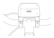
3. Open the clamp (B) on the controller pad and place it in the correct position (it is suitable for handlebar: ∮ 22.2).
