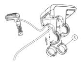
Now place the display on to the handlebar in the correct position, with two M4\*8 screws (D), tighten the display (C the clamps) into position. Torque requirement: 1N.m.
